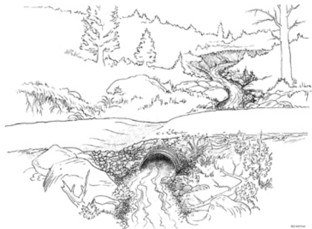
Figure 7-23 This sketch shows an armored overflow dip designed to insure only the loss of some road fill in the event of culvert failure.
