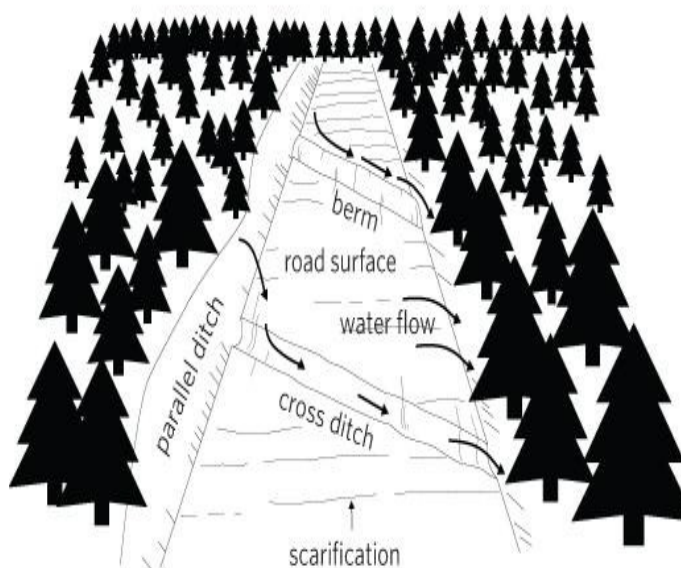
Figure 7-14 Bird's eye view of ditch relief
